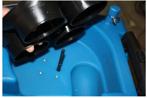
C. Put your left hand into machine to hold feed motor while using your right hand to remove 4 screws
