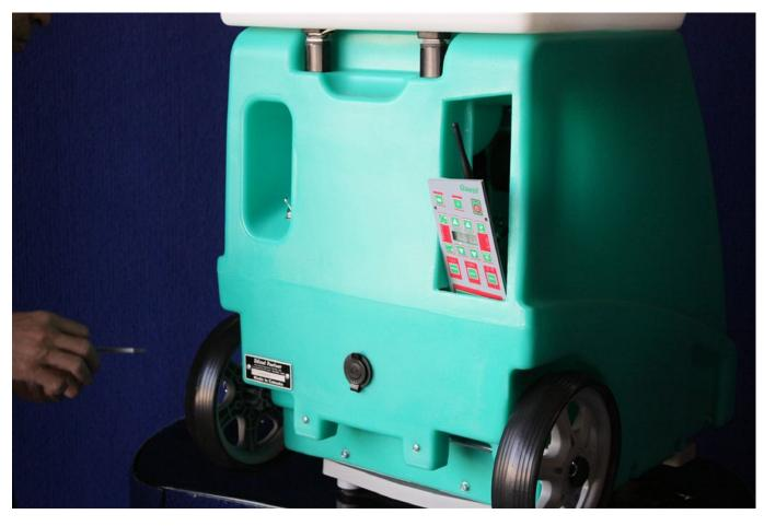
3. Tilt the top of the panel towards you and extra the assembly with all wires connected.
