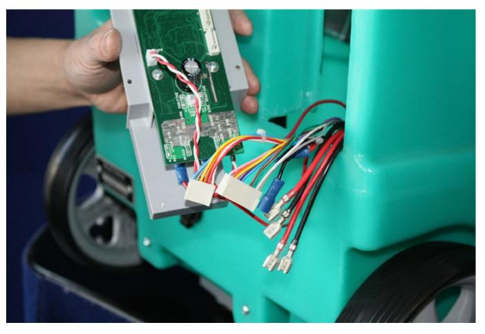
6. The two thick wires connected to the circuit breaker must also be disconnected.
