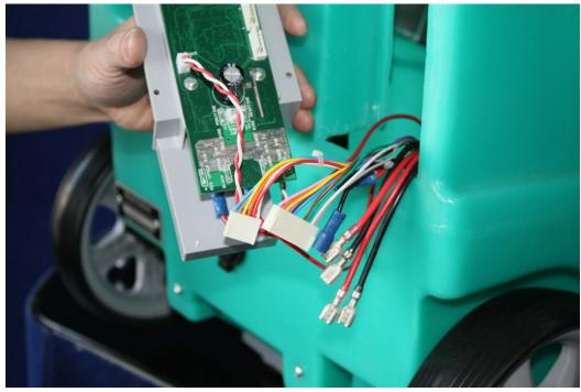
6. The two thick wires connected to the circuit breaker must also be disconnected.
