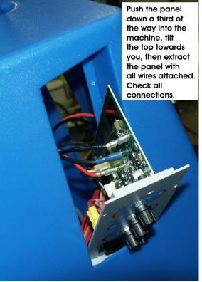
Depending on what you need to do, you can either verify that all connections at the panel are secure, or you can proceed to replace the circuit board.
