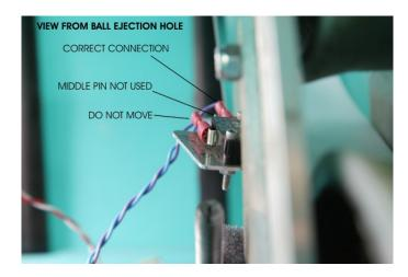
The photo below shows the correct connections at the switch. You will not be able to observe the switch from this angle, so be sure to inspect the connections carefully from the ejection hole.
