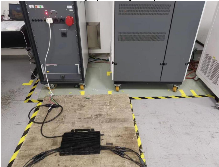
Harmonic, Voltage dips and voltage interruptions test
