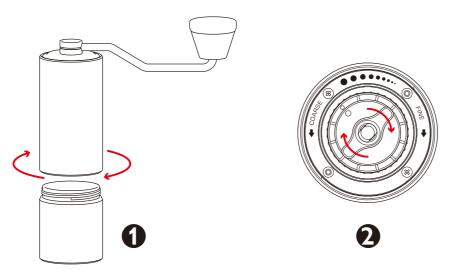
Pull out the container. Set up coarseness by turning the scale at the bottom of the body.
