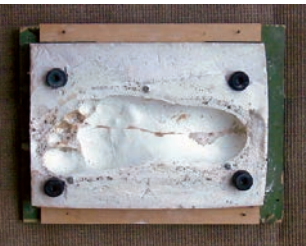
Mold for the first idea of minimalist and five-toed shoe.
