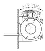
16 equally positioned pin holes ensure seamless clutch transmission and make it easily rotate by 22.5° Increments.
