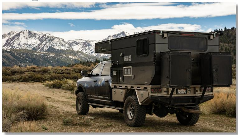
Dry Weight: 1,395 Lbs. Roof/Wall Framing: Aluminum
