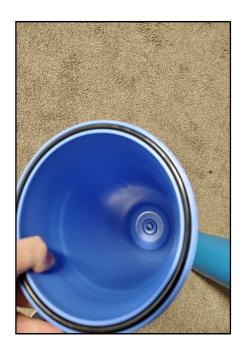
8. Lubricate the O-ring on the filter housing sump and install it. Tighten the filter sump hand tight. That should be adequate. Do not use abrasive tools to tighten the housing or damage may occur.
