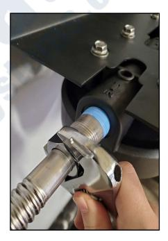
6. Connect the outlet plumbing to the outlet on the filter housing. Tighten with an adjustable wrench.
