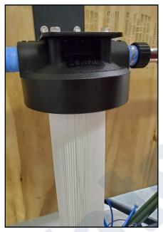
6. Lubricate the O-Ring for the sump and the sump threads with food grade silicone grease.
