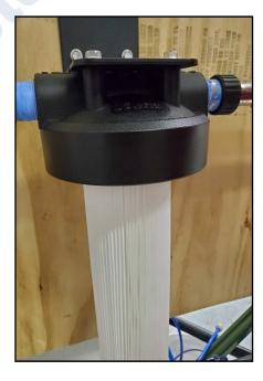
8. Lubricate the O-ring on the filter housing sump and install it. Tighten the filter sump hand tight. That should be adequate. Do not use abrasive tools to tighten the housing or damage may occur.
