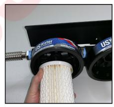
5. Lubricate the O-rings and install the new filter in the filter housing cap.
