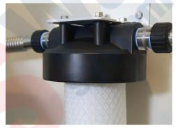
2. Lubricate the O-ring on the filter housing sump and install it. Tighten the filter sump hand tight. That should be adequate. Do not use abrasive tools to tighten the housing or damage may occur.
