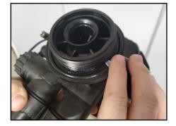
7. Install the upper basket on the bottom of the valve by lining up the tabs then turning the basket clockwise to lock it in place. Place the upper basket over the distributor tube and push the valve onto the tank. Thread the valve on the tank by turning it clockwise. Be sure not to cross thread the valve on the tank.
