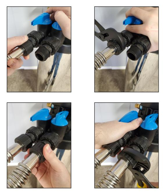
NOTE: All piping should be secured to prevent stress on the bypass valve and connectors.
