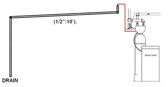
NOTE: A direct connection into a waste drain is not recommended. A physical air gap of at least 1.5" should be used to avoid bacteria and wastewater travelling back through the drain line into the softener.
