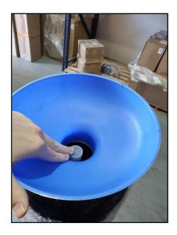
6. Lubricate the distributor O-ring and the outer tank O-ring.
