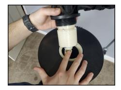
8. Tighten the valve hand tight then snug it further by tapping it with the palm of the hand. **DO NOT** use tools to tighten the valve or damage could occur.
