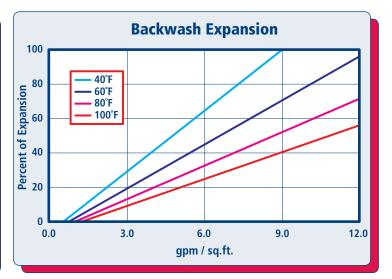
The graph above shows the expansion characteristics of ResinTech *CG10* as a function of flow rate at various temperatures.
