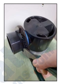
9. Proceed to connect the inlet plumbing to the inlet port of the in/out head.
