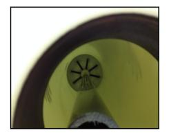
3. Use a piece of duct tape to cover the top of the distributor tube to ensure media does not enter the tube.
