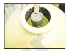
4. Use the funnel provided to pour the media into the tank. The order the media is poured is important. Begin by pouring the gravel media first. Once done, the distributor stack or hub and lateral should be completely covered by the gravel. Proceed to pour the carbon blend media next. A helper may be needed to hold the funnel during the filling process.
