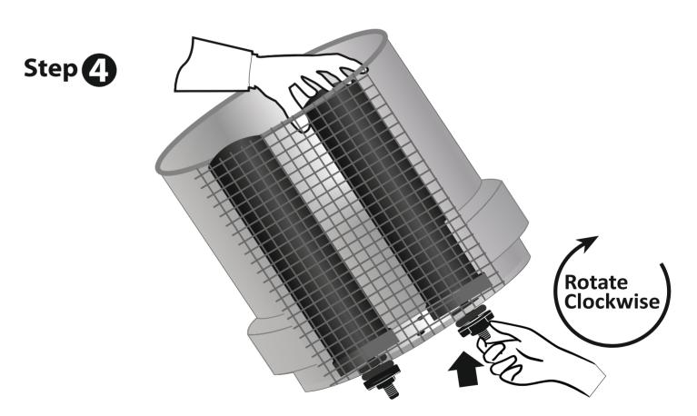
**Important:** Check seals to ensure proper water purification:
