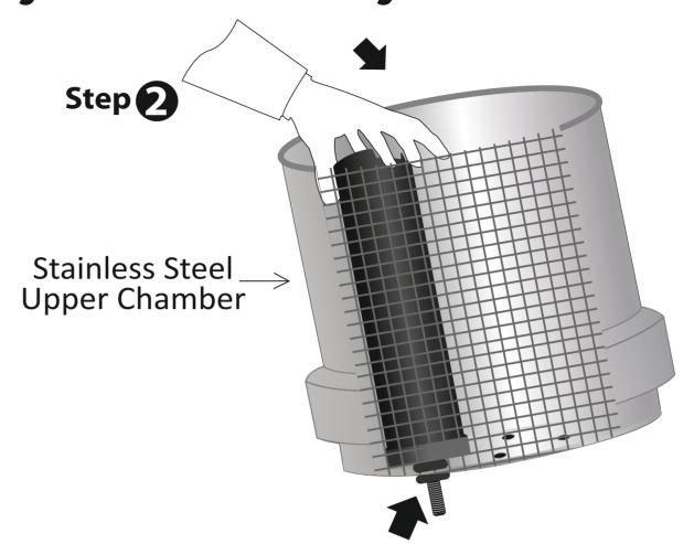
Insert the cartridge thread through any free hole in the upper chamber. The washer should sit flush against base with thread exposed through hole.
