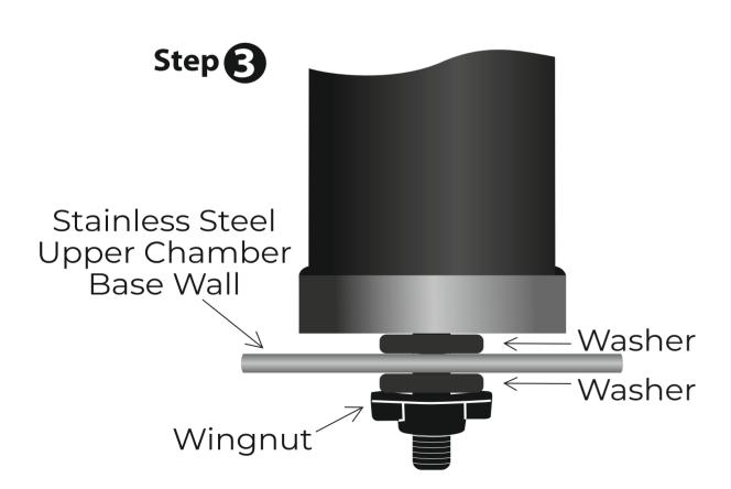
To the exposed thread slide on second washer to base. Securely screw on the wingnut snugly against washer.
