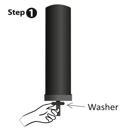
Push first washer along the thread of the carbon filter cartridge.
