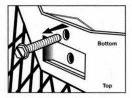
Place the chimney cover upside-down to remove the four screws in the base. Keep the screws — they will be needed later.
