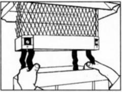
4. Install the cover by placing two legs inside the flue liner no more than 1". Carefully compress the remaining two legs to insert them into the flue liner. With all four legs securely inserted into the flue liner an equal depth, firmly push the cover straight down until the base of the chimney cover is flush against the flue liner or as close as possible. The installation is now complete.
