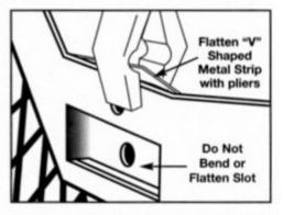
2. The "\( \sigma\)" shaped metal strip inside the base at each corner needs to be flattened. It is advised to use pliers. Do Not Flatten or bend the slot directly below the "\( \sigma\)" shaped metal strip.
