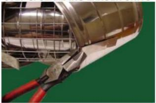
Clamp screens by folding and tightening all three tabs back over top and sides for secure, three-point fit. Repeat process for other screens.
