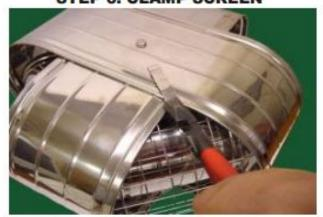
Fold Tab A back over top to clamp screen to Vacu-Stack®. Tighten with pliers. Repeat Steps 1-6 for each of other 3 screens.
