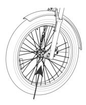
Use a 15mm open-end wrench to tighten the wheel axle bolt to the recommended torque value of 25-30Nm.
