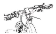
Stand in front of the bicycle, with the front wheel between your legs. Ensure that the handlebar is straight, align the upright with the front wheel, make sure that the clamping bolt of the riser is tightened, and the wheel cannot turn the handlebar before clamping.
