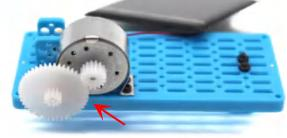
Assemble the big gear to the axle.
