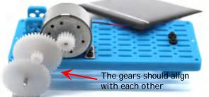
Insert the gear axle to the upper hole of shaft. Fix it with a sleeve.
