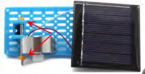
Penetrate the short axle into the shaft. Assemble two sleeves to fix it.
