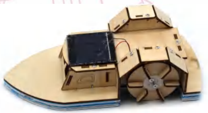
Paste the foam base on the bottom of the boat. Finish and test under the sunshine.
