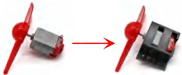
Installation fan blade on motor and install motor base
