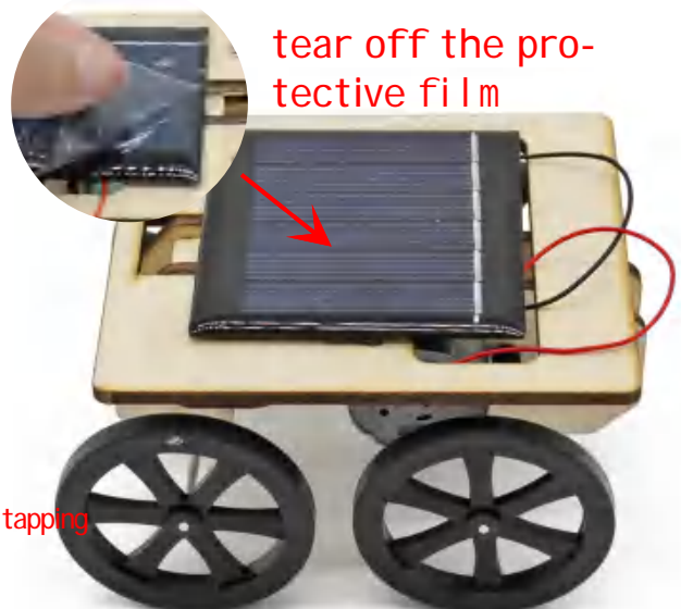
Paste the solar panel
