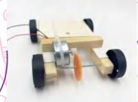
Assemble step 5 to step 4.adjust the position of the big gear and use white glue to paste them.the two gear can not be so tight in case of run not smoothly.
