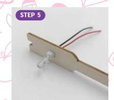
Put the longer wire of the light into the hole connected to the red wire and put the shorter wire into the hole for the black wire.
