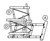
Put the bamboo chair seat support into the hole which located at the bar chair back leg
