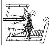
Put the front leg into the hole in the two side support
