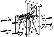
Install the bolts and nuts as per above diagram shown to standard together the bar chair
