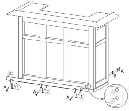
THERE ARE INDICATION MARKS INDICATE WHERE TO AFFIX THE BOLTS TO THE FOOT RAIL. PLEASE DRILL THROUGH THE MARKS BEFORE AFFIX THE BOLTS TO THE FOOT RAIL.
