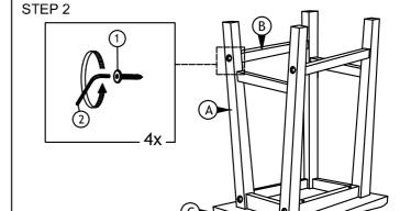
Attach the stool leg(A) with apron seat(C). Do not tighten any hardware completely!
