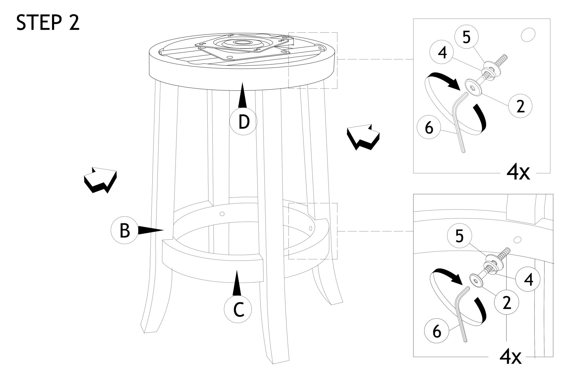
Attach part (B) with part (D) and part (C). Insert each individual hardware as per picture shown. Tighten part (B) with part (D) first, then tighten part (B) with part (C) completely.
