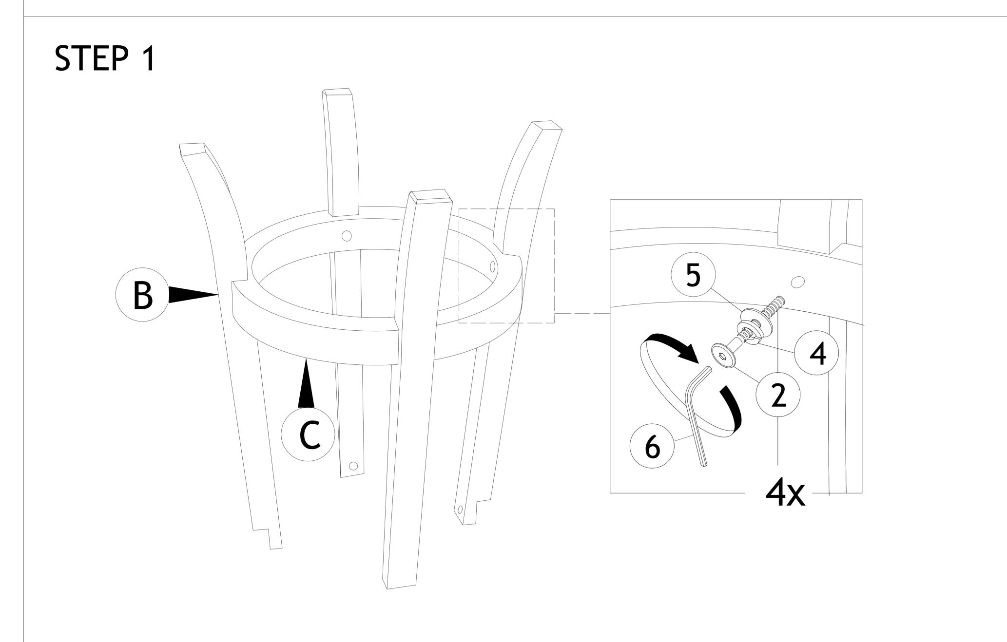
Attach part (B) with part (C). Insert each individual set of hardware as per picture shown. Do not tighten any hardware completely.
