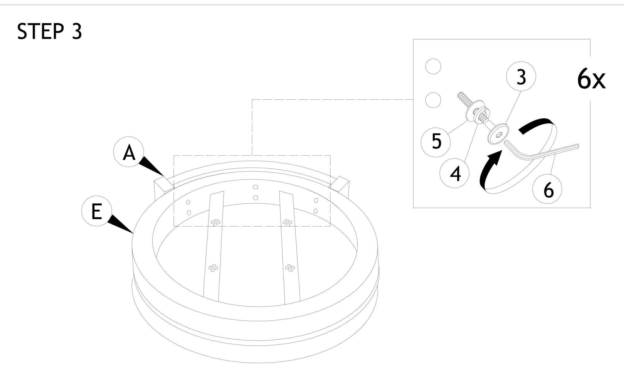
Insert 6 sets hardware first, then tighten part (A) with part (E) after alignment is done.
