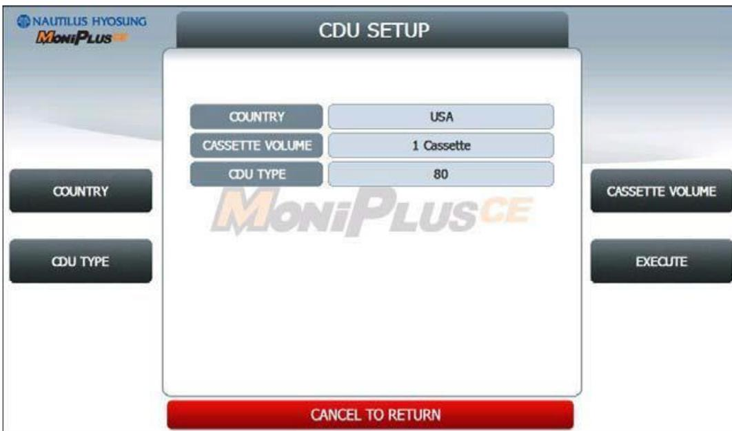
34. Once the CDU Setup has been set correctly, we need to go to Card Reader setup and change it to NH DIP if we have a DIP Reader Installed. If we have an EMV Reader installed skip this step.
