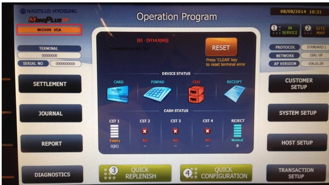
29. If ATM Model Type is incorrect go to System Setup (Function Key #6) > System Control (Function Key #8) > NVRAM Clear (Function Key #8) > Clear All (Function Key #1) > Select Model Type of this ATM > Apply & Clear (Function Key #8) > Yes we are sure (Function Key #1). Then the ATM will count down and reboot by itself.
