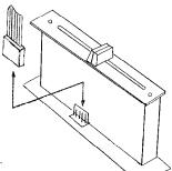
●Insert the connector to the new fader unit.
