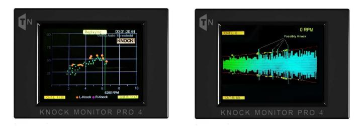
Outside of what the chart shows, you can still identify knock using the waveform view. Look for repetitive spikes in the waveform as is displayed in this photo on the right.
