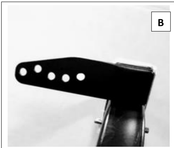
Crossbar setting for rear leaning ROPS.
