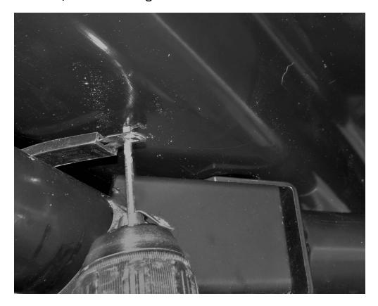
4. Use the washers, screws, and lock nuts to secure the canopy to the loop clamps.
