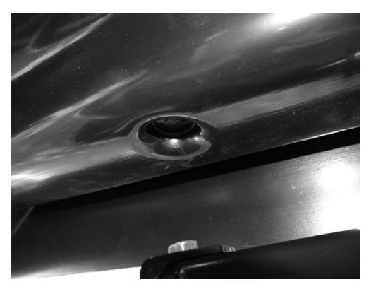
3. Drill pilot holes through the canopy to match the location of the loop clamps. Then drill the 5/16" mounting hole for the bolts.
