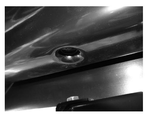
3. Drill pilot holes through the canopy to match the location of the removable straps. Then drill the 5/16" mounting hole for the bolts.
