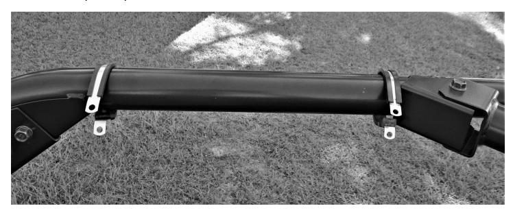
2. Place the canopy on top with the dimples over the rear bolt heads on the ROPS.
