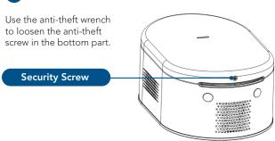
Lift the bottom up and gently push up to remove the complete cover.
