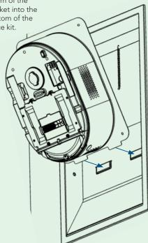
Attach the chain included with the ADA compliance kit to the top rear slot of the protection bracket of the device.
