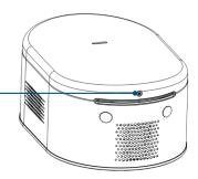
Lift the bottom up and gently push up to remove the complete cover.
