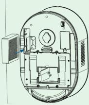
Insert AC filter into the unit box, then insert the unit box into the device.
