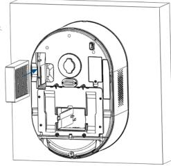
Insert AC filter into the unit box, then insert the unit box into the device.
