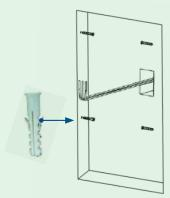
Align the ADA compliance kit to the wall and secure it with 4 wood screws.
