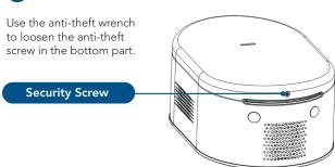
Lift the bottom up and gently push up to remove the complete cover.
