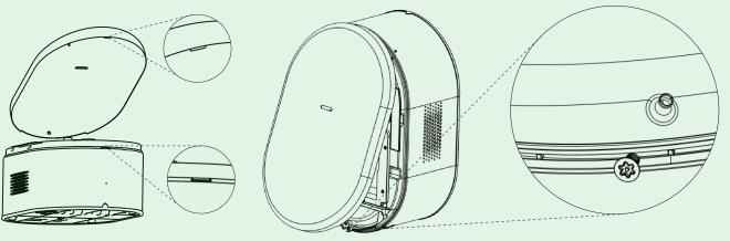
When installing the top cover, first insert the positioning piece at the end of the top cover against the positioning hole of the main unit.
