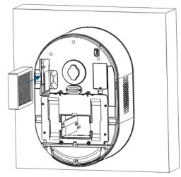
Insert AC filter into the unit box, then insert the unit box into the device.
