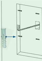
Align the ADA compliance kit to the wall and secure it with 4 x wood screws.
