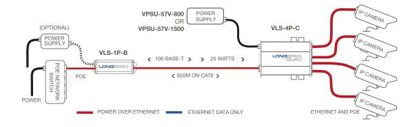
Range is for typical 24AWG Cat5e or 23AWG Cat6, 4-pair UTP.
