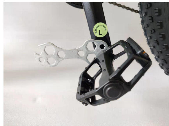
Turn spanner counter-clockwise to fix the pedal L
