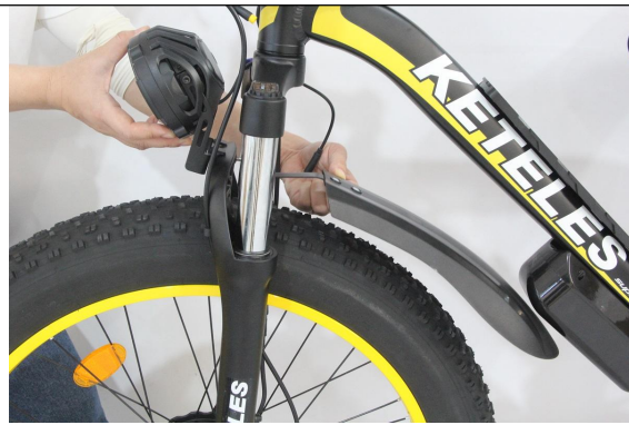
Fix Headlight and fender to the fork brace
