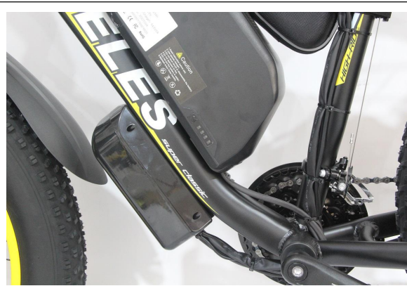
Push the battery downward and lock it
