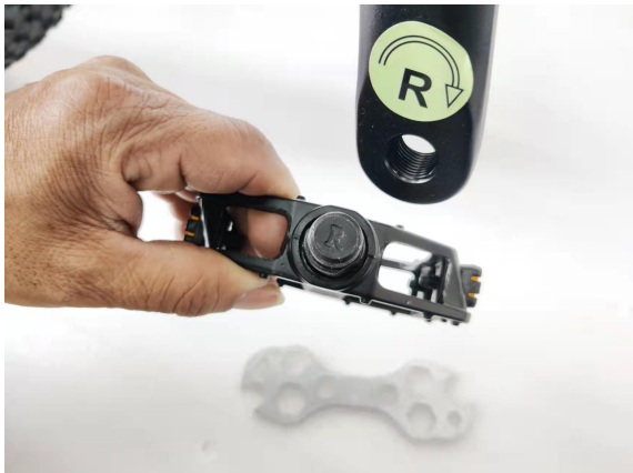
The pedal with letter R should be fixed on the right
