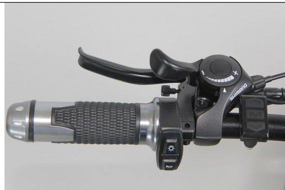
Press button M for 3 seconds to turn on display
