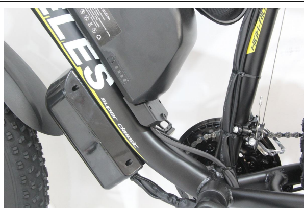
Put the battery on the battery base
