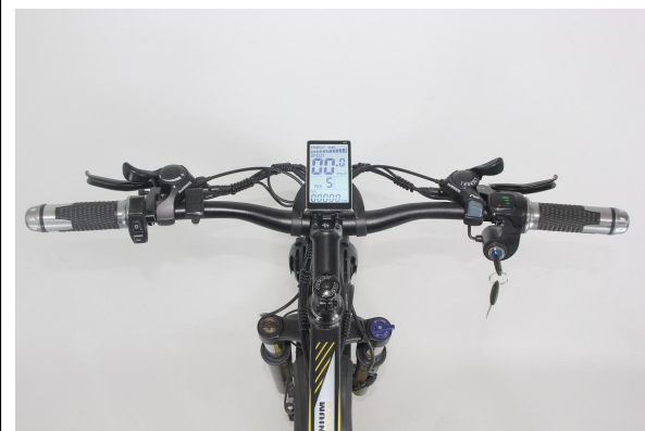
Press button \wedge or \vee can change speed grade .
