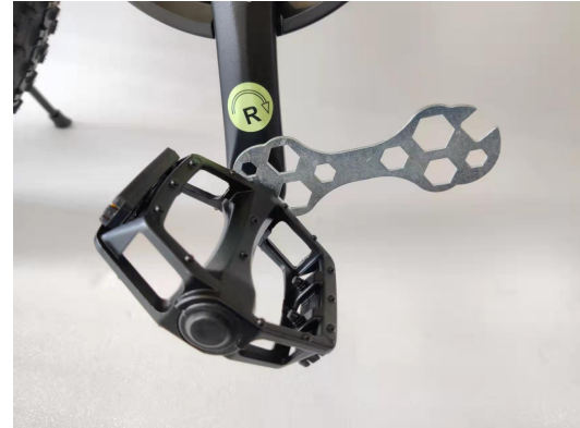
Turn spanner counter-clockwise to fix the pedal L
