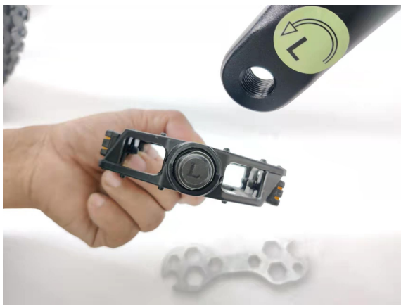
The pedal with letter L should be fixed on the left
