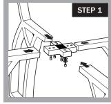
before screwing through leg into "X" connector. Screw in casters and tighten nuts using wrench provided. While assembling, leave screws loose to allow adjustment in cart. Otherwise it can be difficult to get all of the screws in. After cart is assembled, confirm all bolts are tightened, then lift Kamado and set into cart with bottom vent centered between two legs.
