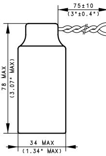
Note: For best performance battery should be mounted in the application in upright or horizontal position.
