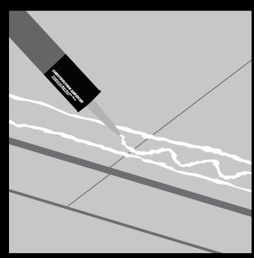
② Apply polyurethane adhesive to the floor between the pencil marks.
