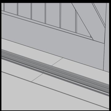
**5** Lower the door onto the threshold trim and allow adhesive to set up overnight.
