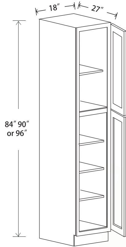
Utility Pantry • WP188427 / WP189027 / WP189627 • One adjustable top shelves • Note: 84" H Two bottom shelves 90" H or 96" H Three bottom shelves • Note: Roll Out Tray kits available for utility cabinets See page 41"
