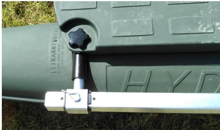
6. Here is a picture of the Back end of the Left side rail (note the hand knob is at the rear):
