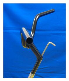
• Again using the 6mm Allen Wrench, tighten the handlebar stem.
