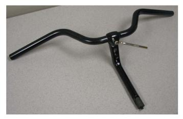
• Place the stem into the rudder tube. Be sure the handlebars are perpendicular to the rudder.
