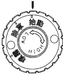
**3** Move throttle lever to low-speed position.
