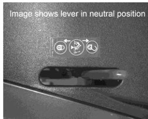
If the lever is in neutral position the motor is decoupled and the brake function is deactivated. Do not park the scooter in neutral position on a slope
