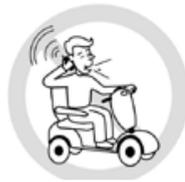
Never use electronic radio transmitters such as radios or mobile phones during operation
