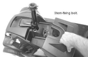
The height of the seat is adjustable; stability may be affected by the center of gravity
