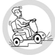
Do not attempt to negotiate obstacles that are higher than the ground clearance value given in the table.
