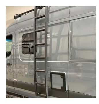
6 - Double check the ladder is still parallel to the caulking seam and tighten the upper 4 bolts.
