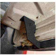
Fasten the brackets to the vehicle and Sliders using the M10 bolts and washers. Spray on rust proofing is recommended on the self-tapping screws.
