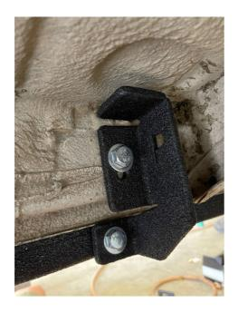
Using a 1/2" drill bit, (a step bit is recommended) drill the holes and install the M10 rivnuts in the rocker panels and in the sliders, being careful not to damage the exterior of the rocker panels.
